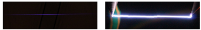
Figure 1: a) Filament induced by a focused 50 mJ, 100 fs laser pulse. b) Guided discharge (15 kV, D = 4 cm, 30 \mu s)
