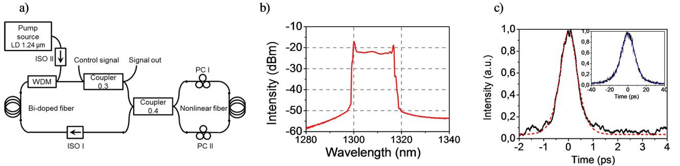
Figure 1: a) – The F8L scheme of the pulsed bismuth doped fiber laser. b) – Spectrum of solitons. c) – Autocorrelation functions of the pulse signal obtained at the output of laser (inset) and after compressor
