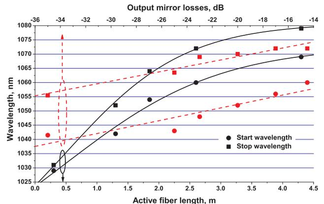
Figure 1: The dependence of the sweeping range on the active fiber length at fixed output mirror losses of -15 dB and on output mirror losses at fixed fiber length of 2.6 m
